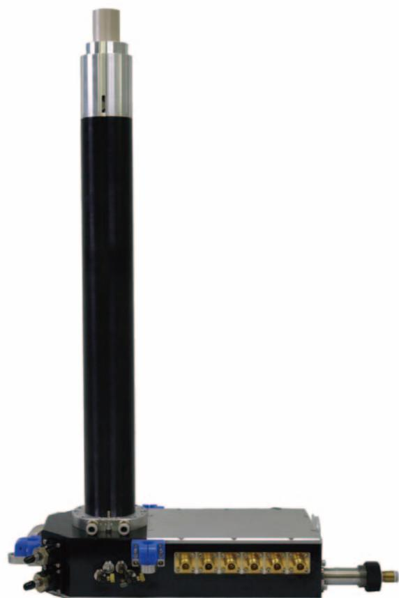
Photo of the external view of a prototype Cryo-Coil MAS Probe for multinuclear measurement.
