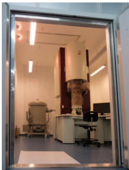
The JEM-ARM300F with double  $C_s$ -correction by JEOL – nick-named the “Grand ARM” – in its shielded and air-conditioned booth. This particular booth is placed inside the hall of a new lab building on a non-vibrating fundament.
